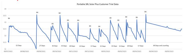
The above graph shows data retriefed from live customer trials, commencing Summer 2022. Where voltage is dictated on the Y axis, and dates on the X axis, we can see the frequency of battery exchanges over an 11 month period. A total of 13 battery exchanges were completed. 'BX' denotes battery exchange.
