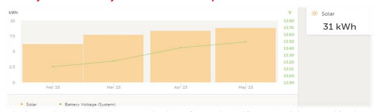
The above graph shows 31kWh solar energy produced over a four-month period from one signal (data retrieved from live customer trials), removing the need to undertake battery exchanges. This delivers a CO2 reduction of 1139.28 Kg, equating to 3.7 Tons over 12 months. CO<sub>2</sub> reduction assumes average site with eight units onsite.
